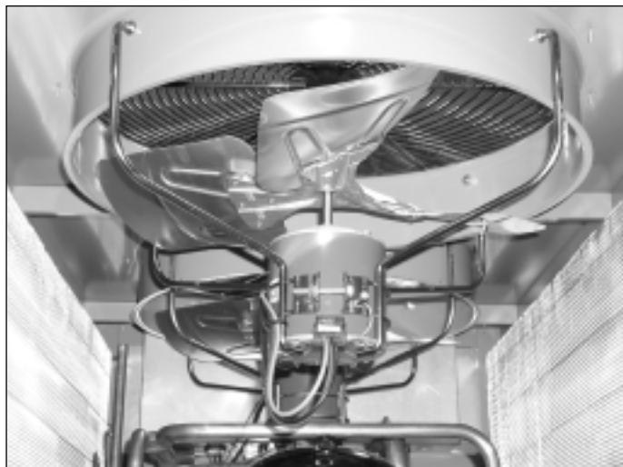
CONDENSER FAN MOTORS —Direct drive, single-phase permanently lubricated “PSC” motors with inherent overload protection.
